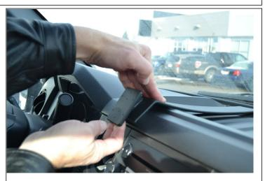
2. While pressing down on the middle section of the ProClip, place your fingers behind the face plate and flex the lower angled edge over the dash over hang closest to you.
