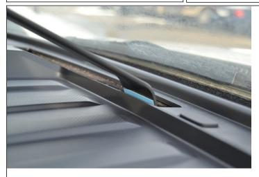
1. Peel off the cover of adhesive tape on the ProClip. Note: The adhesive tape does not leave any marks or damage the dashboard, and is easy to remove.
