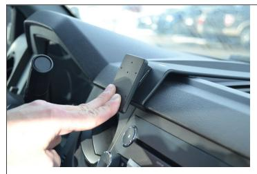
3. Press forward on the face plate to make sure the ProClip attaches securely.
